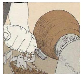
Smooth off the outside with your scrapers. Then, keeping the bowl on the lathe, rub with sandpaper, which will give the wood a gloriously smooth finish.
