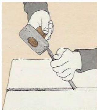
Again using your edging-in chisel, inscribe a V-shaped channel about 1 inch (2 cm) deep between the lines on all four sides. A stone will always break at its weakest point, so be sure your stone has no flaw which will prove weaker than your inscribed notch.
