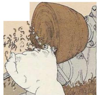
Move the handrest so that you can work on the inside. The unbreakable rule for hollowing wood on a lathe is: begin at the outside and work towards the centre. Start with a gouge, then scrape with round-ended scrapers only, and finally sandpaper it smooth. Remove the chuck from the lathe, unscrew it and fill the holes with plastic wood. Polish the whole thing with beeswax and glue felt on the bottom.
