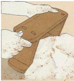
Coat the inside of the mould with sand as you would a cake tin with flour, by dipping in sand and shaking.
