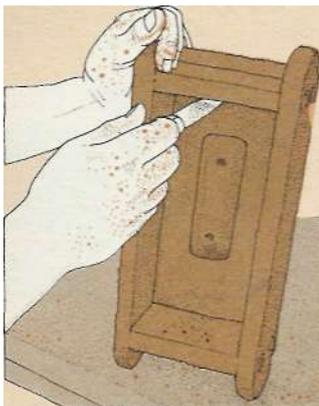
Clean the inside of your mould by scraping round with a knife.
