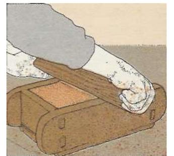
Dip a length of wood in water and use it to smooth over, or "strike", the top surface. Then sprinkle the top with sand.
