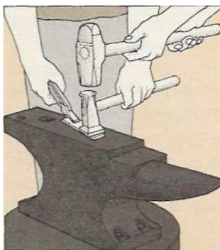
chopping, because its surface is softer and will not suffer damage. The "beak", the long pointed bit, is for working anything that needs a curved edge. To flatten metal, or remove marks made by a hammer or other tool, you should hold hot metal on the face of your anvil with tongs, hold a flatter over it and whack it with a sledgehammer until you achieve the desired effect.
